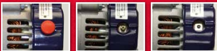
*The active warning light is set as default. To change to inactive, simply remove the screw!*
